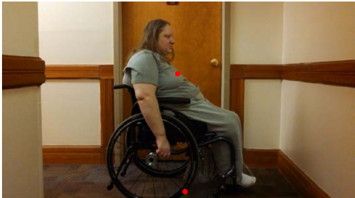
233 234 Photo 2: Anne sitting in an Invacare Crossfire T7A K0005. The rear axle is adjustable and is 235 below her shoulder joint as is optimal for minimizing injury to her shoulders and wrists. Note 236 more of the rear wheel is in front of her hand.
